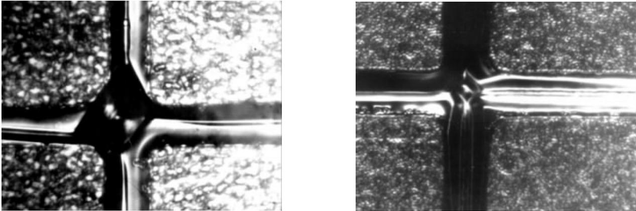
**Figure 1** – Zones cross-section on silicon wafer with (111) (a) and (100) (b) orientation. Entrance surface. 100<sup>x</sup>
