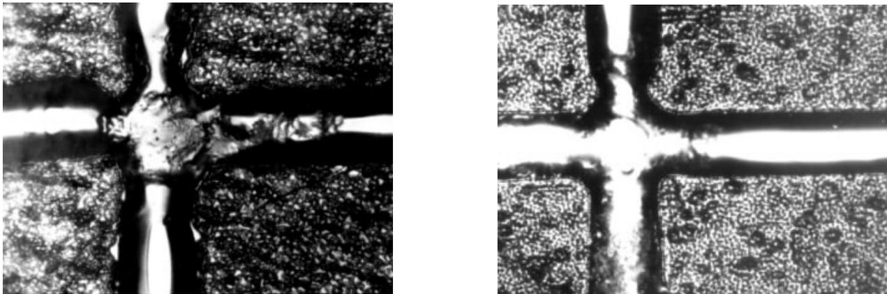
**Figure 2** – Zones intersection on exit surface of a wafer with (111) (a) and (100) (b) orientation after an exit of zones. 100<sup>x</sup>
