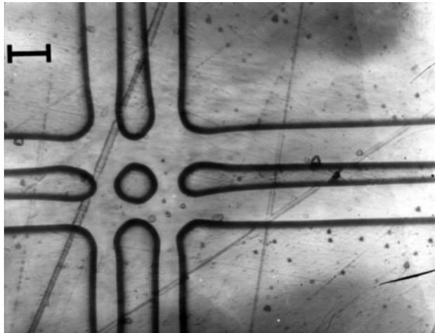
**Figure 3** – Intersection of the doubled zones. Exit surface. 100 $\times$
