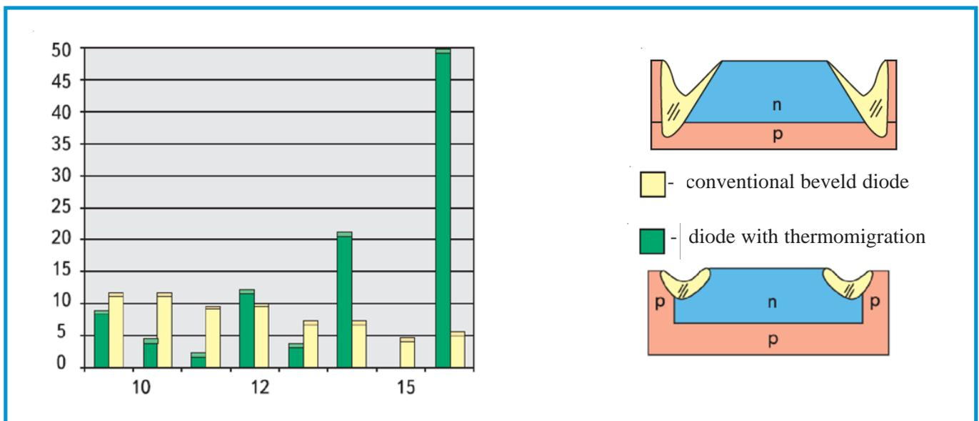
**Figure 4** – Distribution on classes of diode structures Д140-100: with mesa-planar and conventional bevel both passivated by glass.
